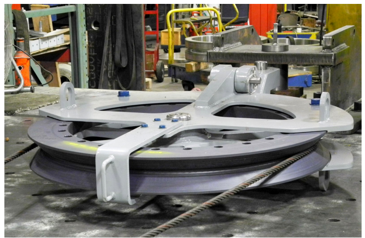
Load Testing of Pivoting Block and Hanging Block for R/V Marcus G. Langseth
