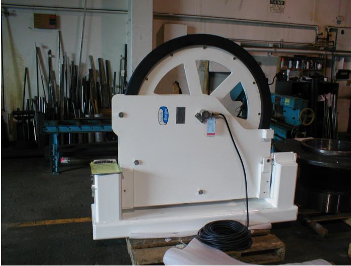
Flag Blocks for 0.680" Wire with Load Pins and Speed/Payout Sensors
